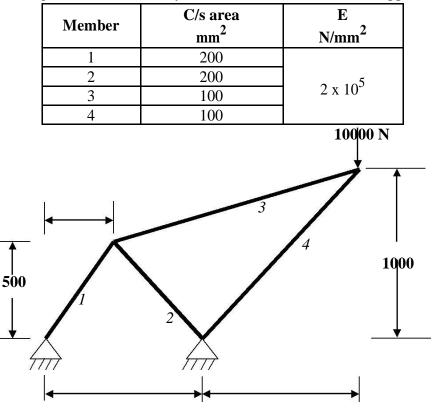
**Prob. 2.** For the given data, find internal stresses developed, Nodal displacement in the planar truss shown in figure when a vertically downward load of 10000 N is applied as shown.
